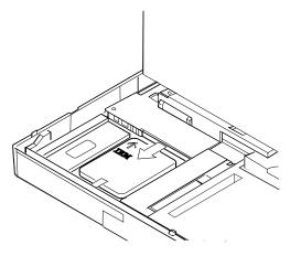
**Warning:** The IC DRAM card is sensitive to physical shock. Incorrect handling of the card can damage it. The eject tape (P/N 53G9318) must be used to remove the card.
